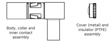
3) Push the cable into the body, as far as it will go. The cable inner conductor will be visible through the hole in the back of the coax body, and should go into the slot in the inner contact.
