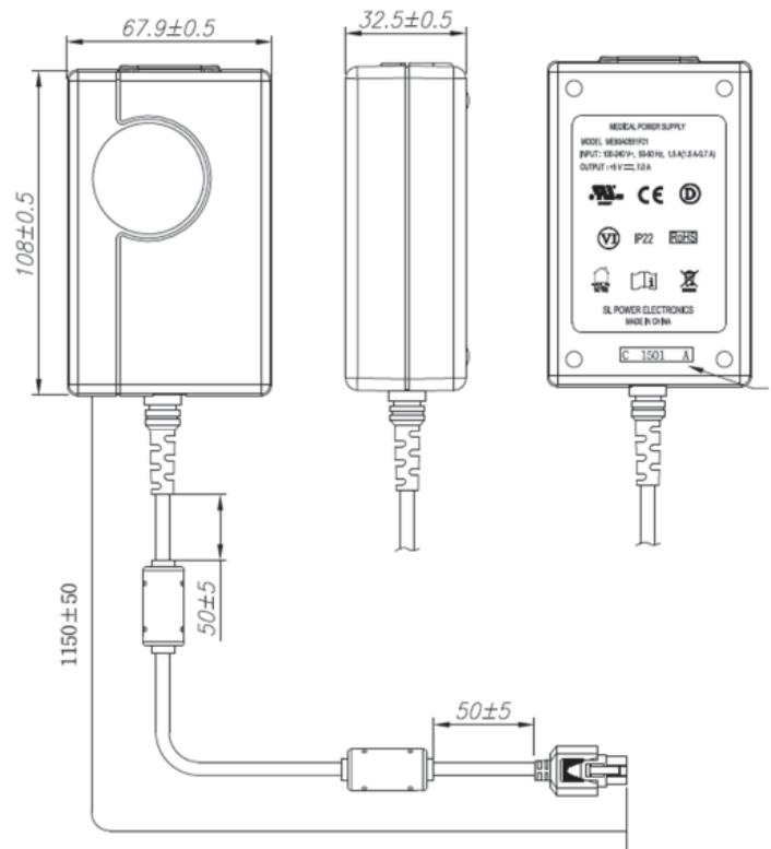
5V Models: Output Connector: 6 pin Molex 39-01-2060 or equiv. Pins 1, 4 = (+), pins 3, 6 = (-), pins 2, 5 = NC<sup>2</sup>
