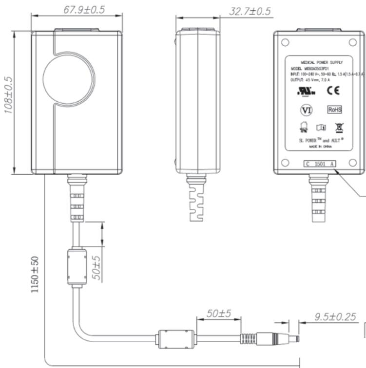
9V through 48V Models: 2.5 x 5.5 x 9.5mm equiv. Barrel Connector, center positive<sup>2</sup>
