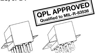
The Series FCA-325 relay is a polarized single-side stable design, where the flux from a permanent magnet provides the armature holding force in the deactivated state, and its flux path is switched and combined with the coil flux in the operated state. This results in appreciably increased contact pressure in both states over that of a spring return nonpolar design. We also manufacture other versions of this relay:
