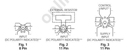
\* If control input is applied when supply input is applied, relay will immediately energize. A 50 millisecond minimum control pulse is required. \*\* Note Input polarity for DC operation. For most reliable operation on AC, connect high side to "+" and low side to "-".
