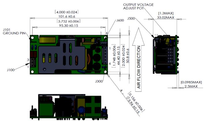
When installing the power supply into the end-product, a non-conductive Insulator should be placed between the unit and any conductive metal chassis or mounting platform.
