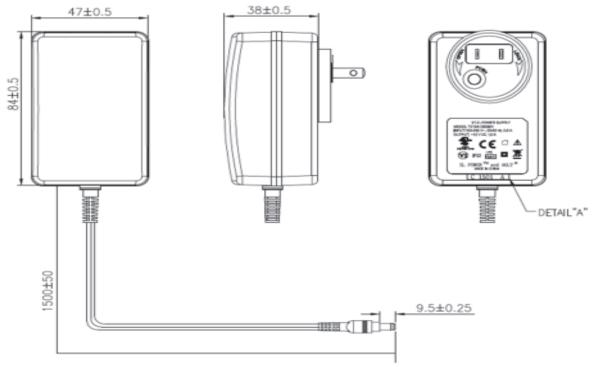
Interchangeable N.A. Blade, 2.5 x 5.5 x 9.5mm barrel connector
