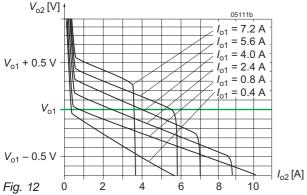
Double-output models with 12 V: Voltage deviation of  $V_{o2}$  versus  $I_{o2}$  for different currents on output 1
