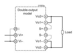
Fig. 2 Parallel-output configuration
