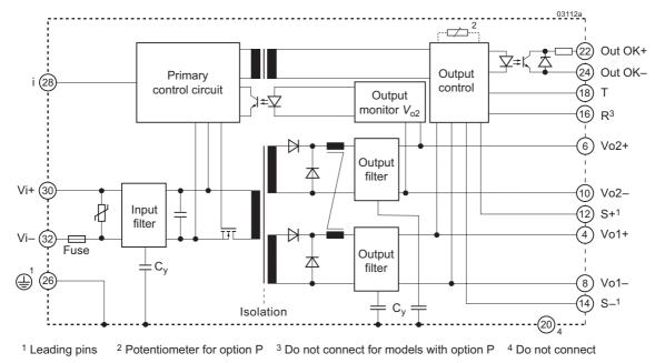
Block diagram of a double-output converter
