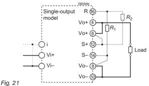
Output adjust using a resistor  $R_1$  (to lower Vo) or  $R_2$  (to increase V<sub>o</sub>).
