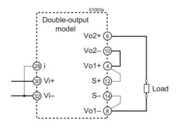
Fig. 3 Series-output configuration
