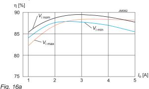
Efficiency versus input voltage and current per output (BQ2320)
