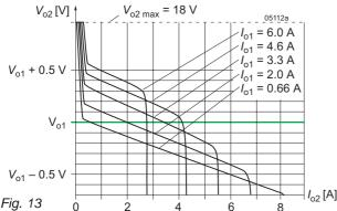
Double-output models with 15 V: Voltage deviation of  $V_{o2}$  versus  $I_{o2}$  for different currents on output 1
