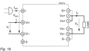
Definition of input and output parameters
