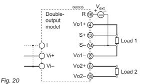
Output adjust using an external control voltage Vext.
