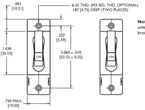
**Note:** Tolerance ± .015 [.38] unless noted. Dimensions in brackets [] are millimeters.
