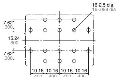
Tolerance:  $\pm 0.1 \pm .004$ Schematic (Bottom view)
