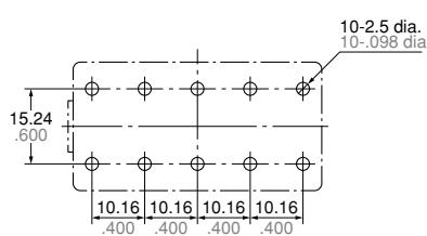
Tolerance:  $\pm 0.1 \pm 0.004$ Schematic (Bottom view)
