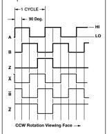
NOTE: Index location is displaced 180° (mechanical) on second output with dual output option.
