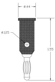
MATERIAL: PLUG BODY- BRASS PER ASTM B16
