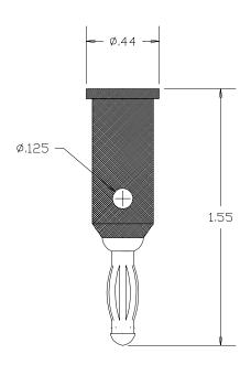
MATERIAL: PLUG BODY- BRASS PER ASTM B16 SPRING- BERYLLIUM COPPER HANDLE- ABS, COLOR: 12-RED
