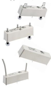
Recently approved by UL, very high isolation voltages (up to 10kV) are achieved through the use of high vacuum reed switches with either Rhodium or Tungsten contacts and make these relays suitable for high reliability applications, such as cardiac defibrillators, test equipment and high voltage power supplies.
