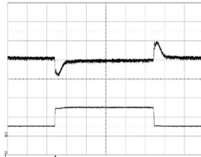
Output voltage response to load current step- change (9,5 – 28,5 – 9,5 A) at: T_{ref} = +25^{\circ}C , V_I = 53 V , C_o = 3,8 mF
