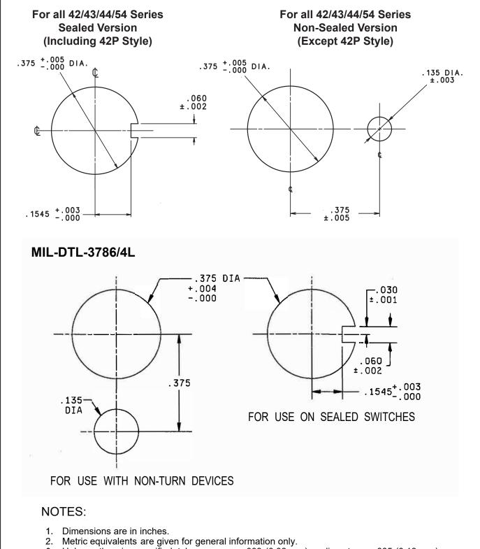
3. Unless otherwise specified, tolerances are  $\pm$ .003 (0.08 mm) on diameters,  $\pm$ .005 (0.13 mm) on all other dimensions, and  $\pm 2^{\circ}$  on angles.
