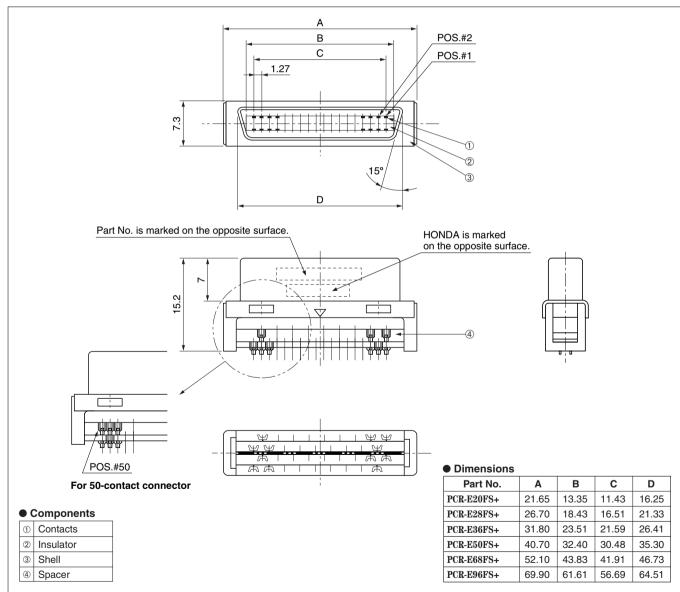
Mating connectors: PCR-E series PCB-side right-angle through hole type or SMT type connector
