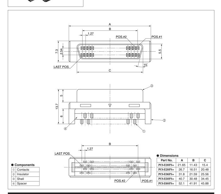
Mating connectors: PCS-E series through hole type male connector for PCB
