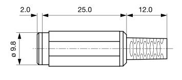
Cable diameter max. 4.0 mm
