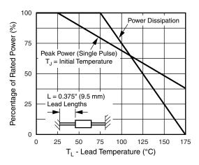
Fig. 2 - Power Derating Curve
