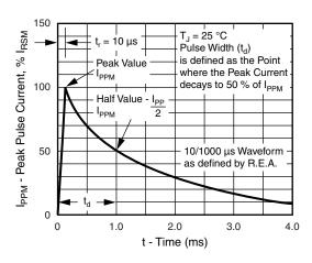
Fig. 3 - Pulse Waveform
